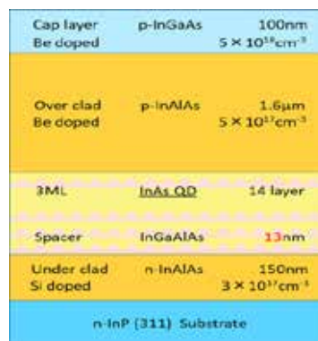
Fig 1. Cross section of 1550nm InAs/InGaAlAs QD wafer on InP (311)B substrate.
