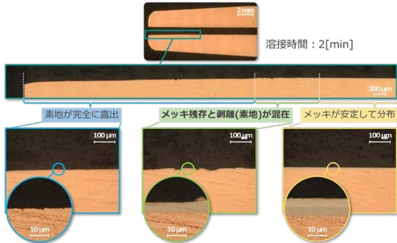
Fig.3 Ni-plating wear on the Ni plated Cu contact tip around the top of a contact tip.
