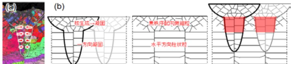
Fig. 2 (a) Solidification in keyhole mode melt pool and (b) schematic diagram of microstructure formation with keyhole mode melt pool.
