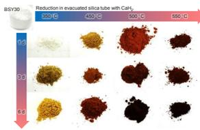
Fig. 1 Appearance of CaH<sub>2</sub>-reduced BaSn<sub>0.7</sub>Y<sub>0.3</sub>O<sub>2.85</sub> samples.
