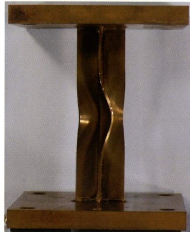
Compression test on cross-section of the column at high temperatures (500 degrees Celsius)
