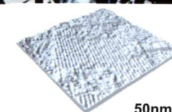
50nmx50nm In situ PLD-STM system equipped with LEED/AES for studies on oxide surface nano-structures. The atomic structure of an anatase \text{TiO}_2 (1x4) film surface was investigated by STM.
