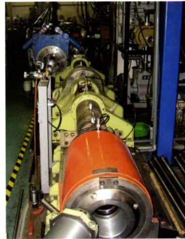
Two-stage light gas gun can generate a velocity up to 4 km/s.
