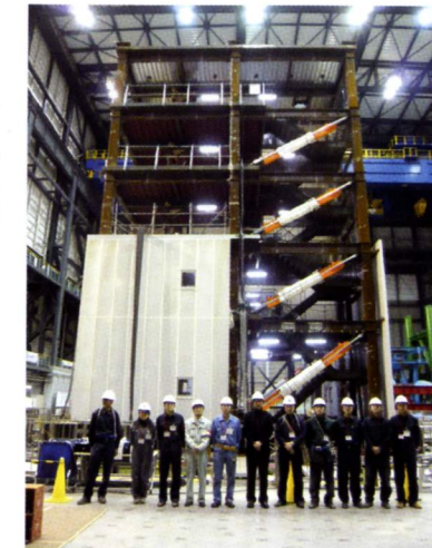
Full-scale Test of 5-story Building with Dampers Using World's Largest Shake-table at E-Defense
