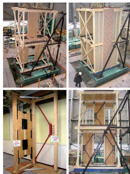
戸建て住宅制振構造の開発と実験 Development and Test for Wooden House with Passive Control System
