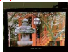
12" AMOLED driven by glass transistor (2008, Samsung)
