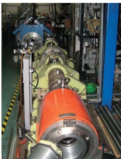
飛翔体を秒速4kmに加速できる二段式軽ガス銃 Two-stage light gas gun can generate a velocity up to 4 km/s.
