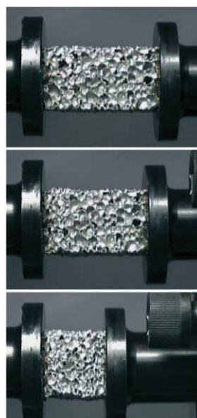
アルミニウム発泡材の圧縮変形挙動の観察 Observation of Deformation Behavior of Aluminum Foam under Compression
