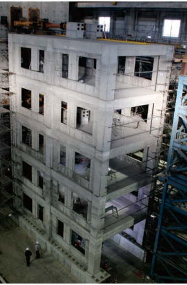
Resiliency of five story buildings tested at Building Research Institute (Tsukuba) •Resiliency of reinforced concrete residential buildings were studied
