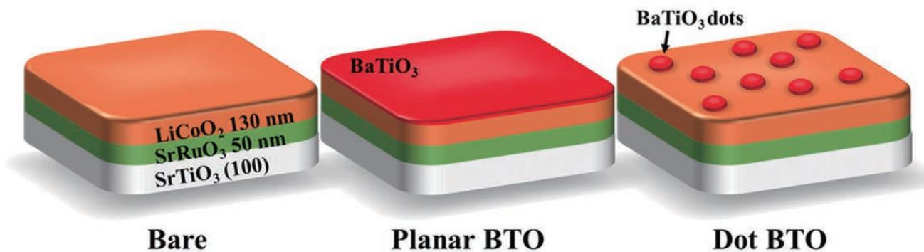
**Modeled structures of LiCoO<sub>2</sub> cathode system in Li-ion battery**
