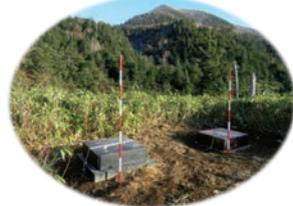
Temporary seismic and geodetic station
