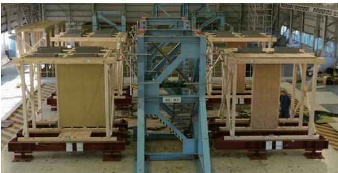
In the 2016 Kumamoto earthquake, major earthquakes attacked multiple times. We research on methods to simulate earthquake response under such severe conditions, as well as technologies to enhance safety level through the application of passive control devices.
