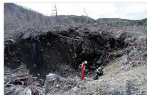
Soil gas sampling at a new vent formed during the 2018 eruption
