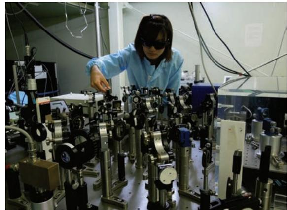
**Femtosecond time-domain interference measurement system**
