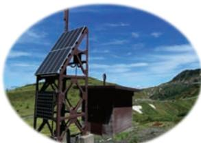
Borehole-type tiltmeter and seismometer station
