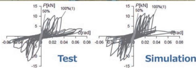
We conduct experiments to verify the behavior of various elements that support the structural safety of wooden buildings (e.g., columns, walls, floors, roofs) to evaluate their performance, and to develop design methods. Evaluation methods of structural performance, and monitoring method for measuring deformation of structures.
