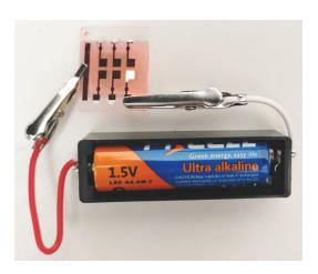
Organic light-emitting diode is operated by a 1.5 V battery.
