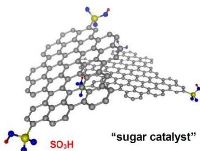
An amorphous carbon consisting of nanosized graphene sheets (1-2 nm) with large amounts of SO<sub>3</sub>H group
