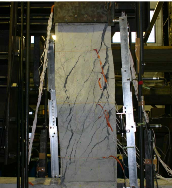
Loading test of reinforced concrete column
