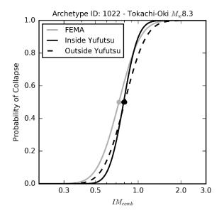
Figure 8. Collapse fragility functions for three groundmotion sets computed using spectral acceleration
