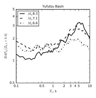
Figure 5. BAF<sub>Sa</sub> with respect to period for varying magnitude earthquakes.
