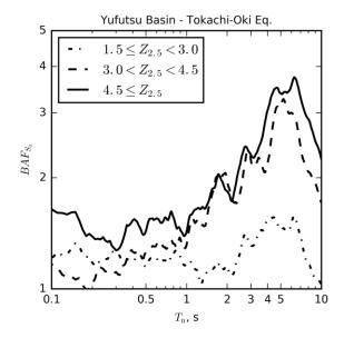
Figure 3. Median  $S_a$  with respect to period for recordings binned in terms of  $Z_{2.5}$  ranges.
